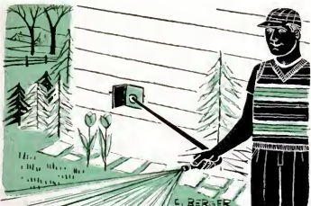
GARDEN HOSES ON AUTOMATIC REELS installed inside the basement. They'd pay out or reel in hose like the extension cord on some appliances.— S. P. Jacobus, Fairfax Station, Va.
